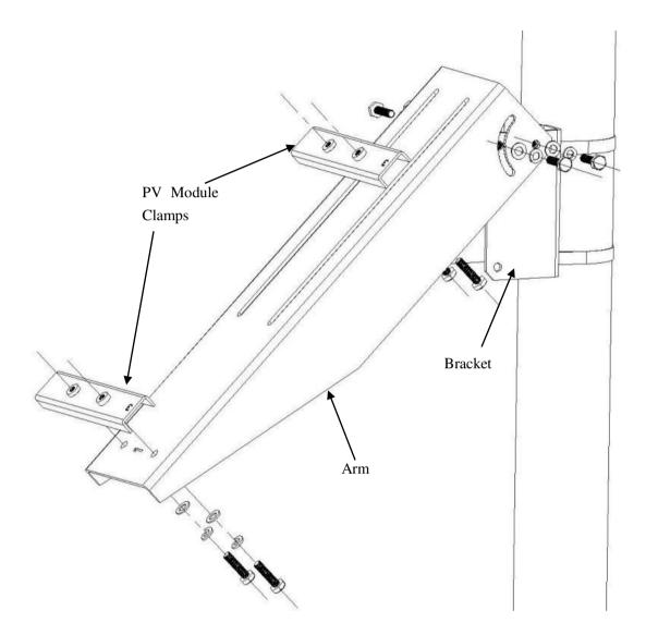
Solartech Power Side-of-Pole Mount support solar panels:
