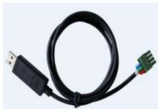
The USB to RS-485 converter is used to monitor each controller on the network using Solar Station PC software and update the firmware. The length of cable is 1.5m. The CC-USB-RS485-150U-3.81 connects to the MC1.5-5.08-2L port (8<sup>th</sup>) on the controller.
