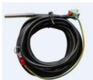
Acquisition of battery temperature for undertaking temperature compensation of control parameters, the standard length of the cable is 3m (length can be customized). The RTS300R10K5.08A connects to the RTS port (10<sup>th</sup>) on the controller.
