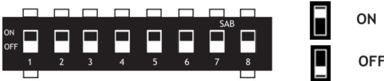
DIP-switch 5 is used for the MPS mode selection.
