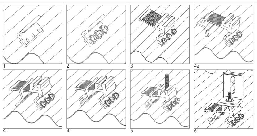
\*Note- It is recommended that the installer assemble and check one complete CorruSlide assembly on the roof panel for fit prior to removing release paper or installing screws. This will provide an indication of approximate fit \*
