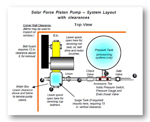
Observe minimum clearances for inspection and maintenance, as show. Bolt the pump directly to a strong, firm surface, NOT on on rubber pads. Expect traces of water and oil leakage at the rod packing.
